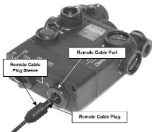
Figure 3.6 Installation of Remote Cable Switch
